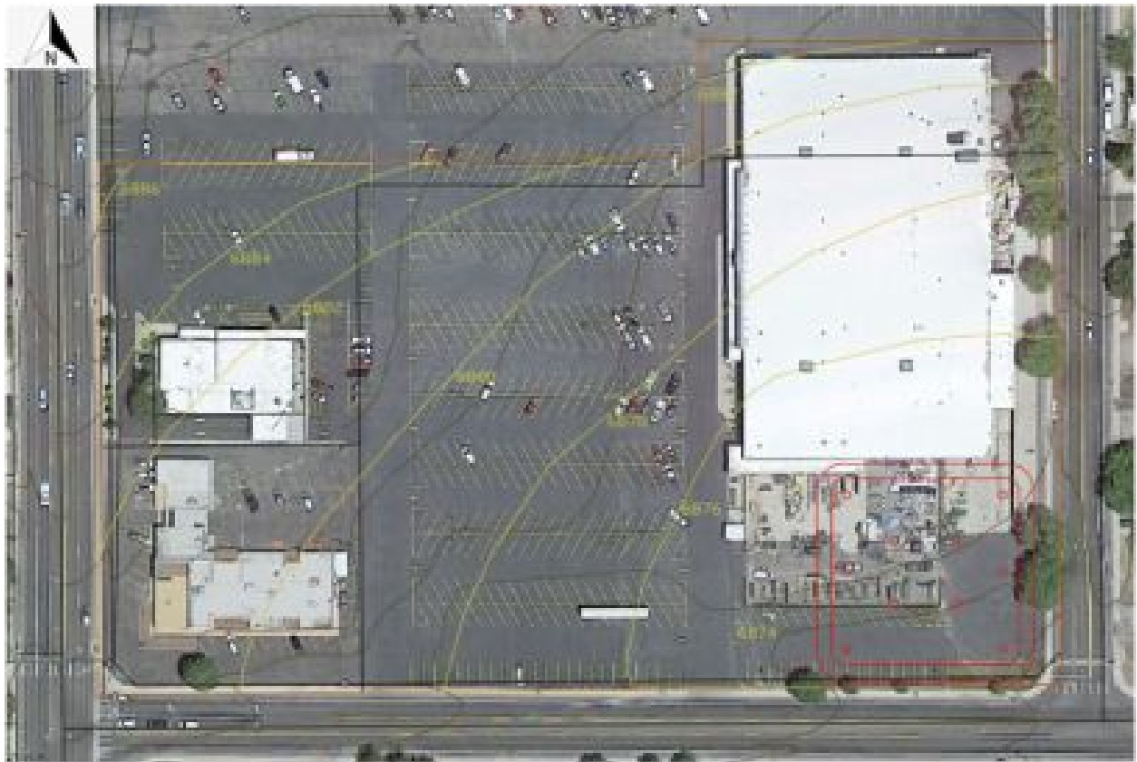
Figure 4.6: Plan of Topography, Retention Basin, and Drywells in Relation to Existing Parcel
